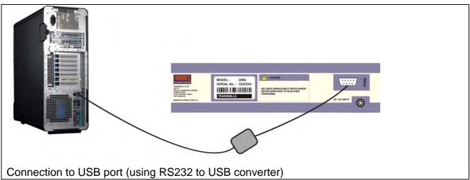
Once connected, using the PC the resistance value should be sent to the 2090 to set the output. The command MUST be terminated with a carriage return (ASCII character 13), for example :
