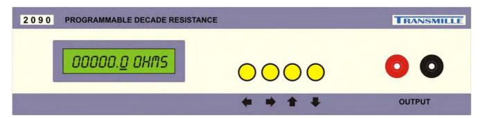
To set up a resistance, simply select the digit required using the left / right cursor buttons (move the cursor to the required digit), the use the up / down buttons to select the required number.
